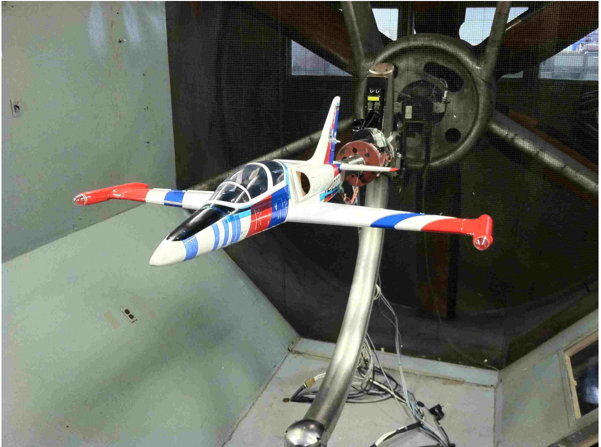
Fig. 1: Photograph of the aircraft on the free-to-roll rig in the wind tunnel.
