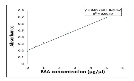
Figure 2.12. Bradford assay calibration curve for Bovine Serum Albumin (BSA) standard solutions. Absorbance values at 595 nm for five different concentrations of BSA were plotted and the best fit line was calculated in excel. The linear equation (x = protein concentration, y = absorbance value) was used to calculate the concentrations of the proteins in tissue homogenates.
