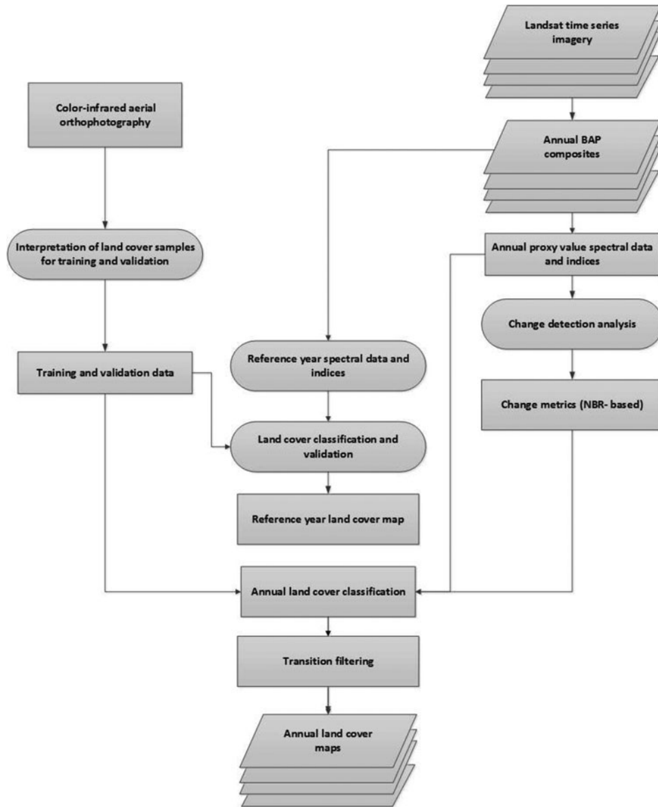
FIG. 1. A flowchart of the overall approach for the annual land cover classification.
