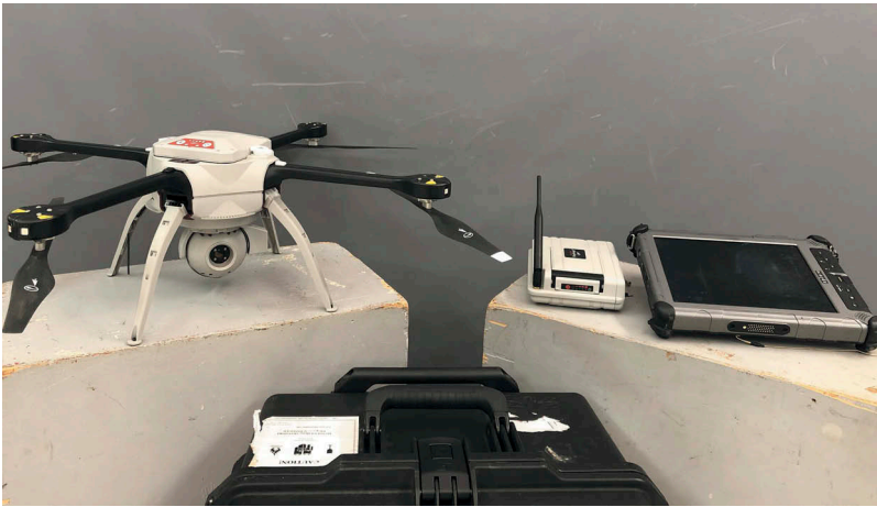
Figure 3. Aeryon Labs Skyranger UAV system equipped with the SR-3SHD payload (left), base station and tablet (right).
