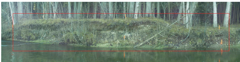
Figure 2. A panoramic photo taken along Whiteman Creek with the Leica Multistation MS50. The red outline indicates the extent of the scanned streambank. The orange stakes on the streambank were used as ground control points for the UAV survey and for manual transect measurements. Additional stakes were placed closer to the stream to aid in manual measurements.
