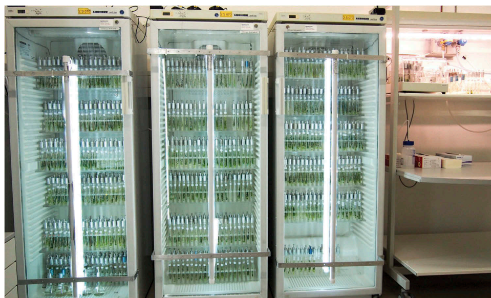
Figure 1. Stock cultures of CCCryo strains from cold locations are maintained in commercial fridges with glass doors for external irradiance at a temperature of 1–5°C. At the top right a small heated box for thermophilic cyanobacteria and red algae cultured at 35°C is visible, next to it are agar slants and culture flasks for isolates that prefer room temperature for growth.
