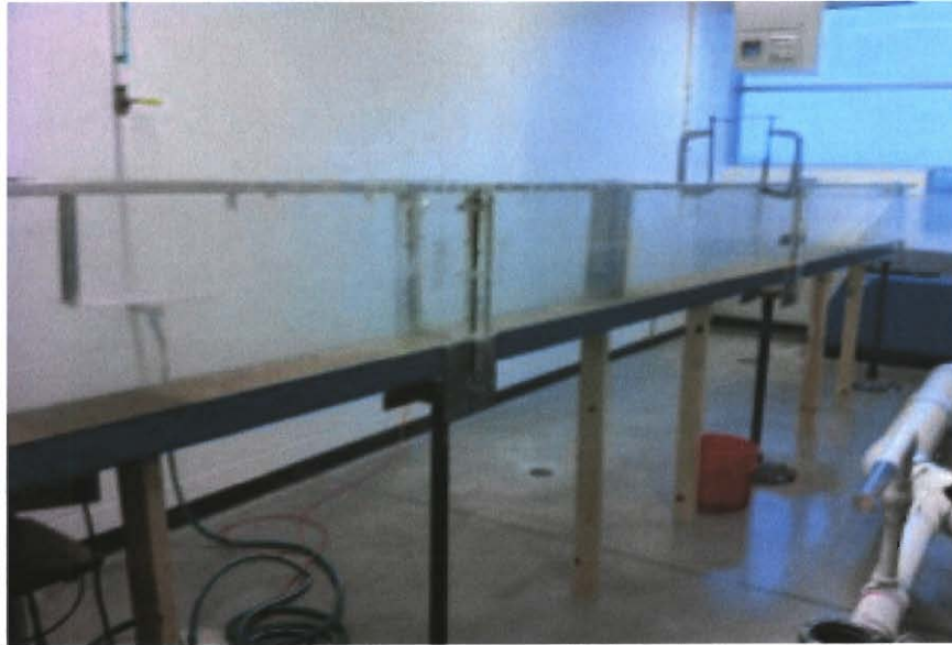
A.4 2x4 legs added to steady the tank
