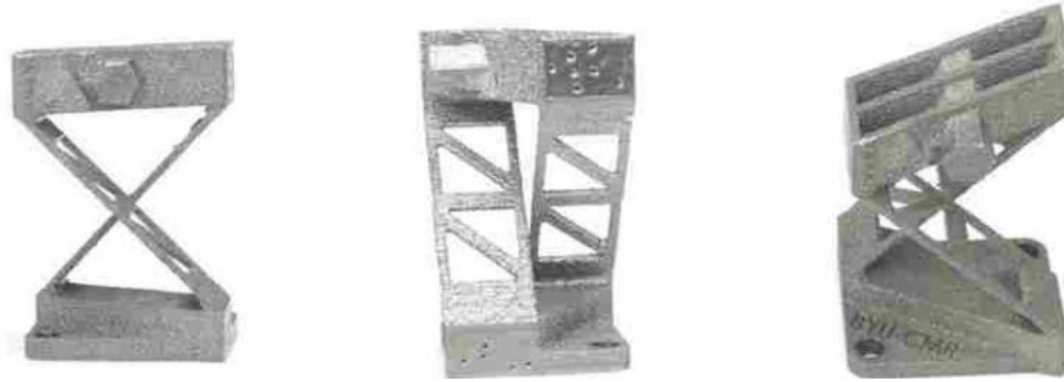
Figure 1.6: A cross-axis flexural pivot designed and built with lattice flexures to reduce the effective width, and thus the stiffness of the joint. It should be noted that although the actuation effort will be reduced with such designs, changes to the effective width of a flexure do not increase its range of motion.
