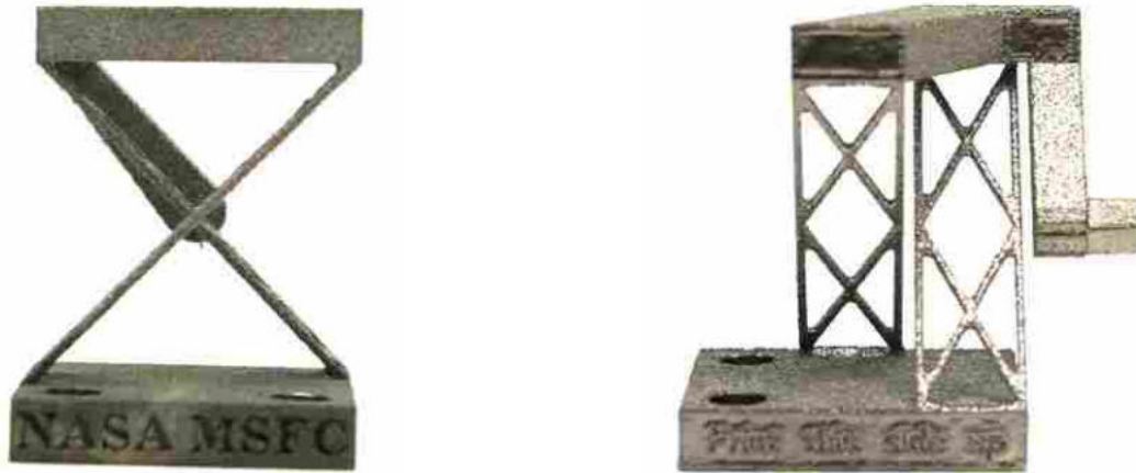
(a) Front view of cross-axis flexural pivot (CAFP) made with lattice flexures.
