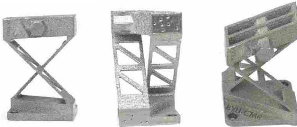
Figure 5.2: A 3D printed titanium cross-axis flexural pivot with an early lattice flexure design.
