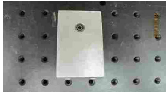
(b) Balance pivot - essentially this is a piece of angled aluminum inset with a small bearing.
