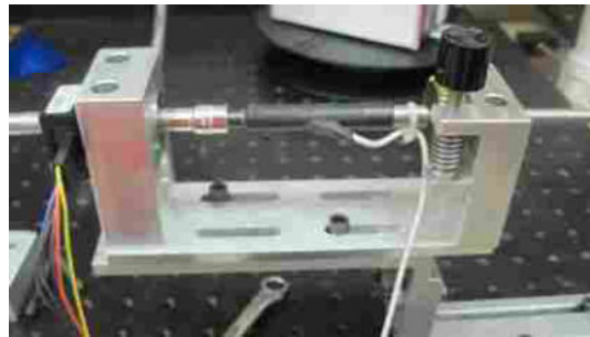
(c) The worm-wheel and pillow block are mounted to a slotted plate so the whole assembly can slide forward or back.
