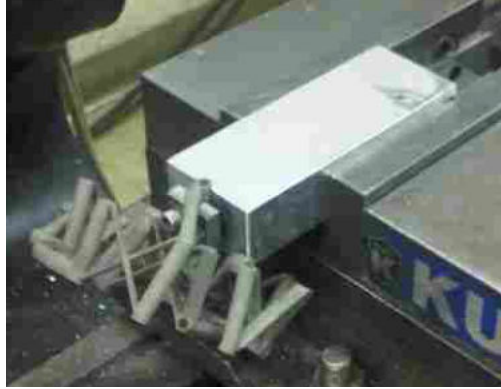
Figure 2.5: The 2 DOF pointer mechanism in fixture for removal of powder and supports from inside a split-tube flexure.
