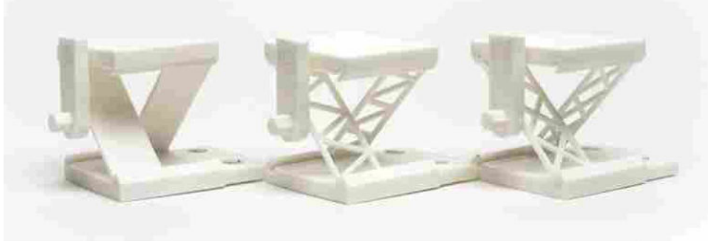
Figure 5.9: Cross-axis flexural pivot prototypes used in the measurement of lattice flexure stiffness.
