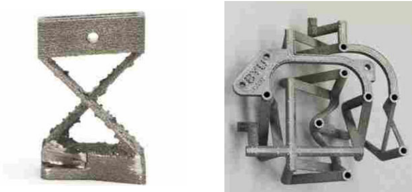
Figure 2.2: Cross-axis flexural pivot and 2 DOF pointing mechanism used to compare FEA and analytical models to measured stiffness.
