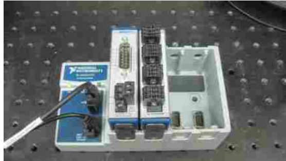
Figure E.7: Plug the modules into the DAQ chassis. Where they go doesn't matter, but keep track of which is where.
