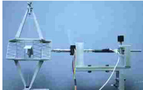
(d) Measuring the stiffness of a statically balanced lattice-flexured cross-axis flexural pivot.
