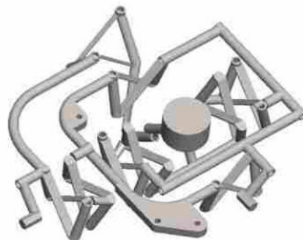
(b) The same mechanism, redesigned with n = 2 for joints along one axis. Also incorporated is an angular offset to reduce center shift to near zero at 15^\circ rotation.
