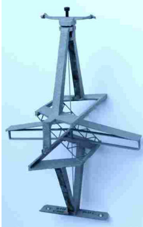
Figure 7.11: Printed titanium flexure.
