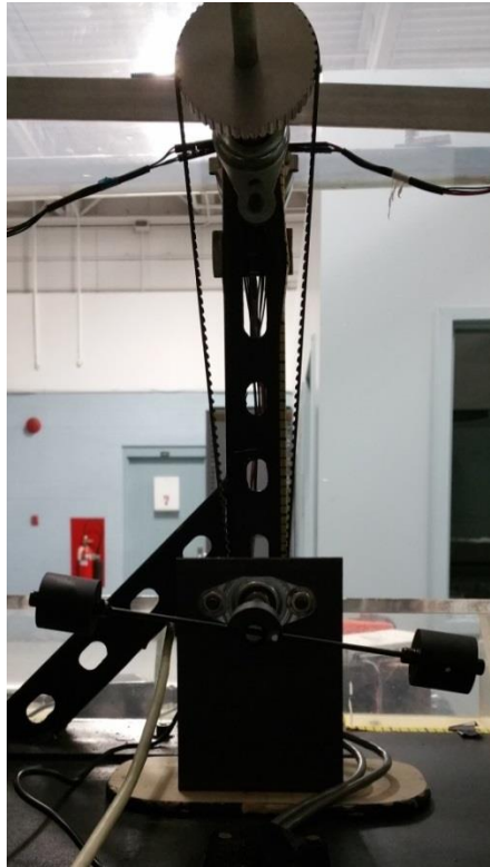
Figure 58: Pendulum setting of the device.
