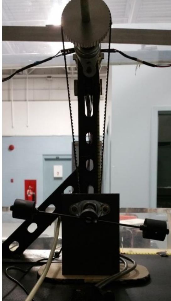
Figure 124: Pendulum photogrammetry target point setting for calculating mechanical power.
