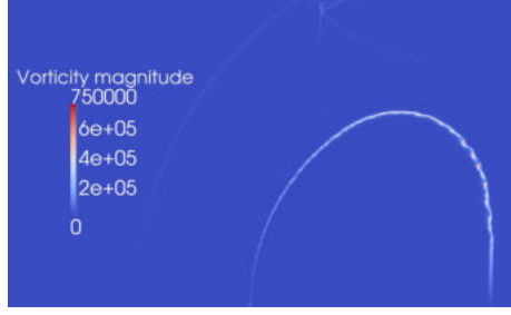
Figure 48: Vorticity magnitude at t = 102 \mu s with 320 \times 40 elements for a cylindrical Helium bubble.
