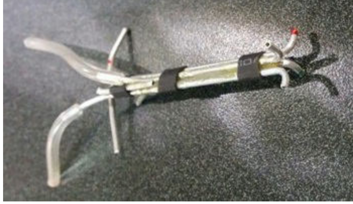
Figure 6.3: Two-pair differential pressure probe set providing radial and vertical velocity components after conversion.
