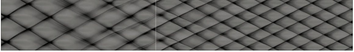
Figure 52: A numerical sootfoil for a gaseous detonation seeded with 0.25 percent by mass of potassium. The maximum magnetic field is B_x = 2000 T . The cellular structures clearly indicate an alteration in the detonation dynamics.
