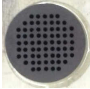
Fig. 3.1.1 Sintered ferrite sample with holes drilled.
