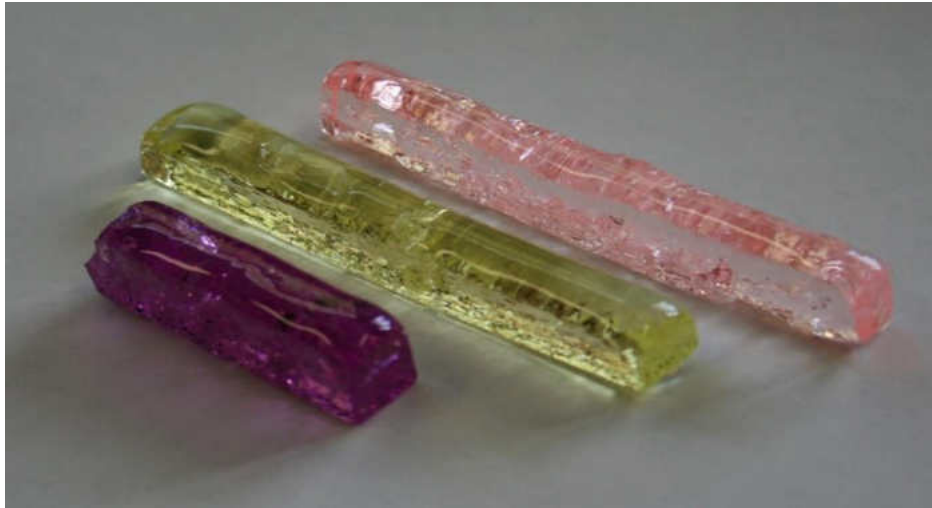
Figure 3. 3: Pr(green), Nd(purple) and Er (pink) doped sodium phosphate glasses.
