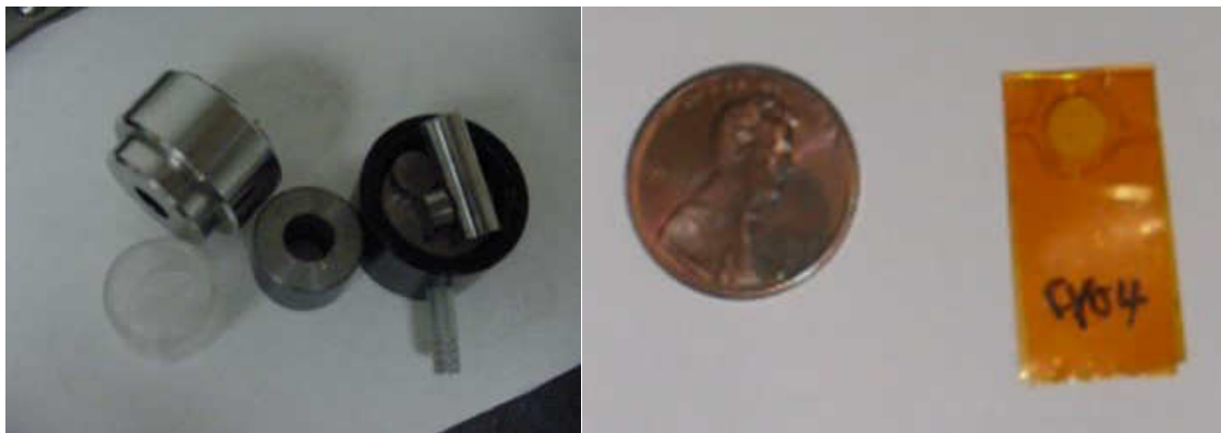
Figure 15. A pelletizer (left) [16] and a prepared ZRLS glass absorber covered with Kapton tape for the XAFS measurement (right).
