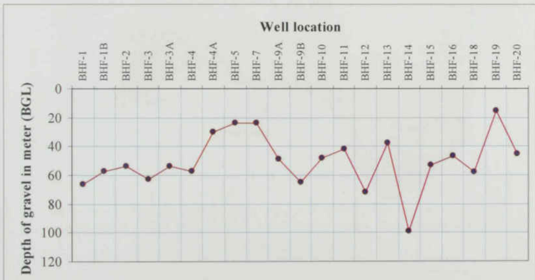
Figure 3.5. Variation of gravel thickness in selected boreholes.
