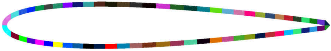
Fig. 21. Decomposed Delaunay subdomains for NACA 0012 Airfoil
