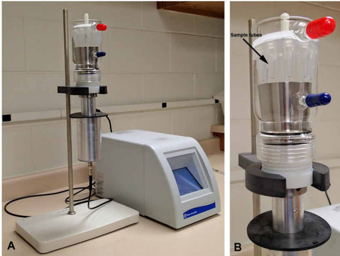
Figure 9. Model 705 Sonic Dismembrator (A) with a 3 inch Cup Horn attachment (B) for simultaneous indirect sonication of 8 samples.
