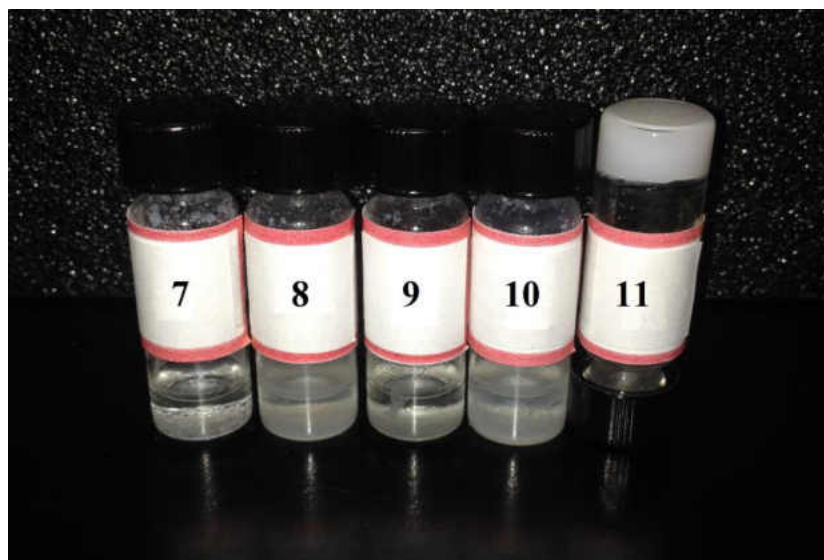
Figure 9. Carbamates 7-11 at 20 g/L ( 2.6 \times 10^{-2} M) in n -dodecane.
