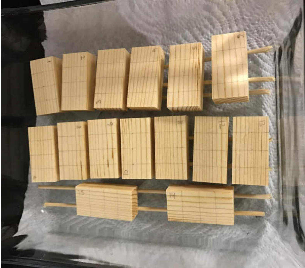
Figure C. 1. Ponderosa pine wood samples (5.0 × 2.5 × 1.5 cm 3 ) dipped in the radiolabeled Woodlife solution and placed on wooden skewers to dry for 24 hours.
