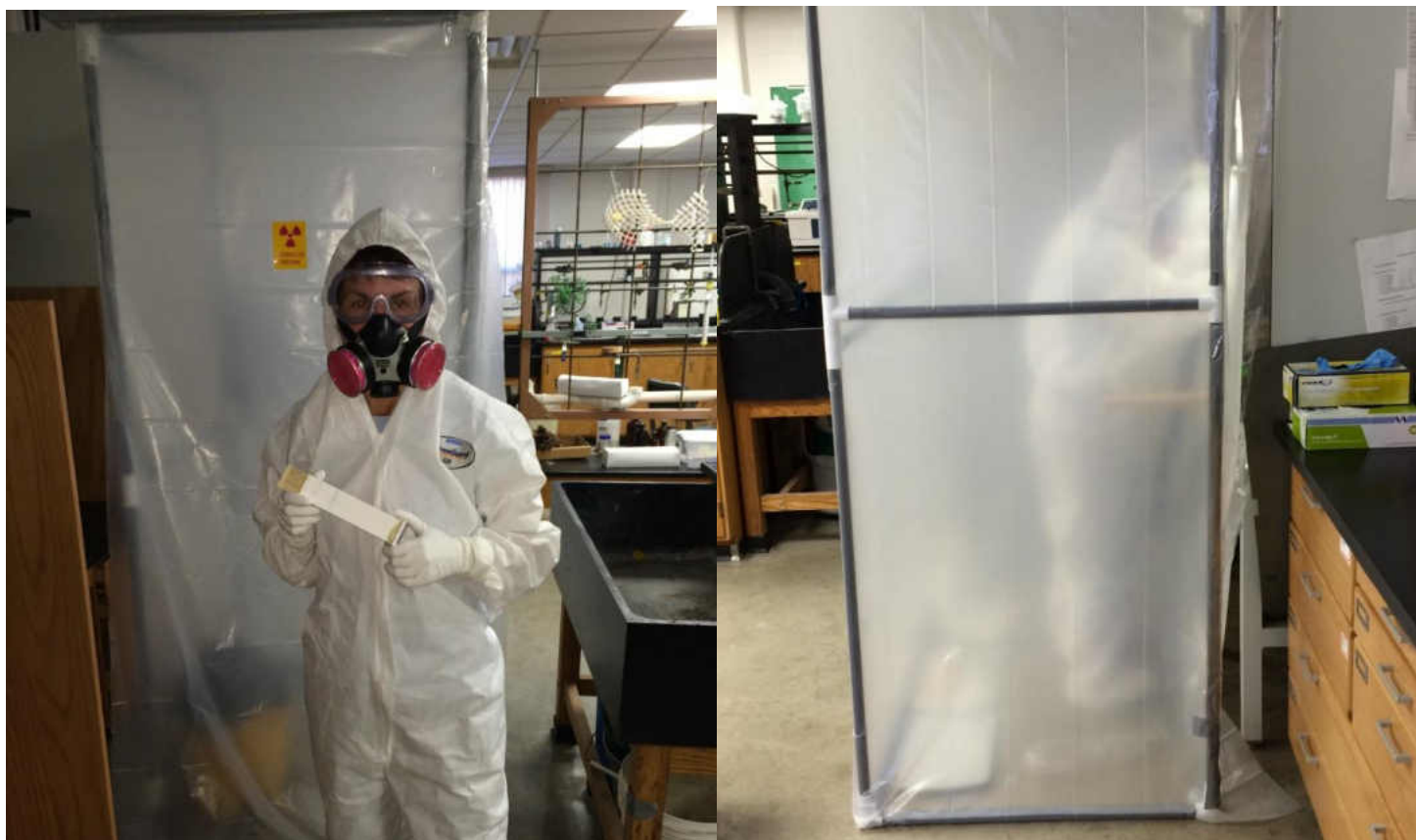
Figure A. 4. Protective hood enclosure to eliminate ^{14}\text{C} -wood dust contamination. The enclosure contained two chambers separated by a plastic sheet. Entrance to the first chamber is shown on the left, while the second chamber attached to the hood is shown on the right.
