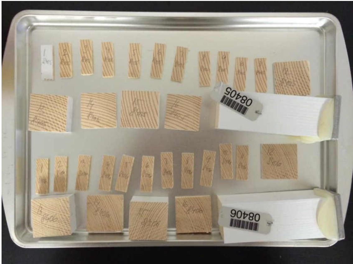
Figure B. 1. Cutting of “T” wood sections with a band saw into 2-mm wide wood slices (#1–12, 14, and 16).
