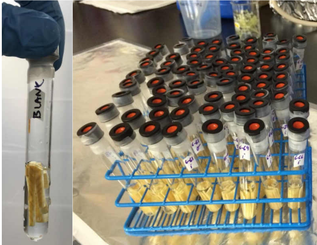
Figure A. 5. Glass tubes containing smaller wood pieces (cut with a blade) and 3.5 mL of acetone.
