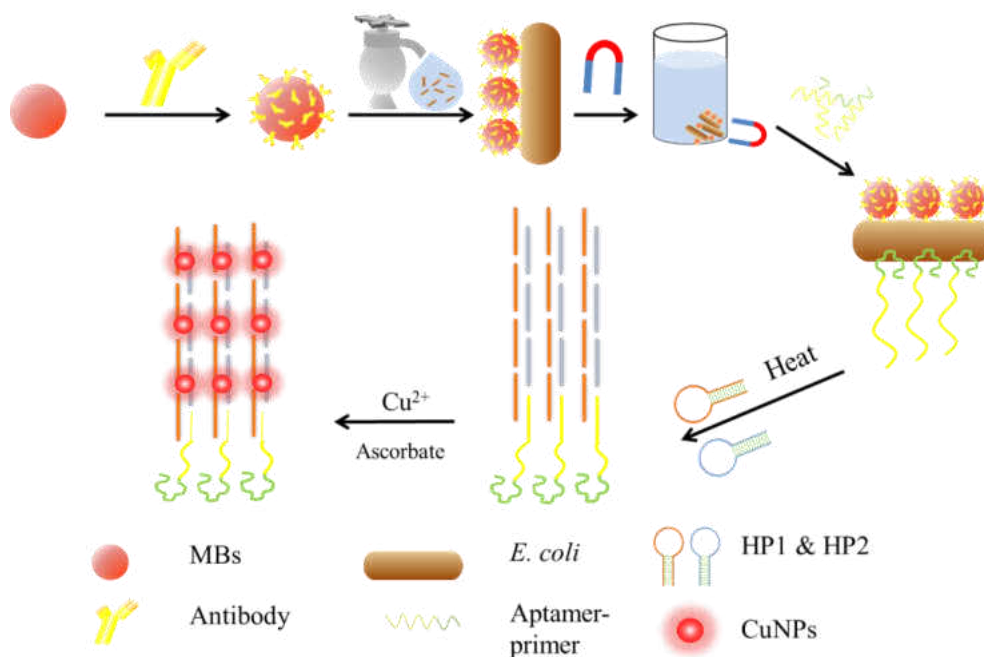
Scheme 3. Scheme for the detection of E. coli using dsDNA-templated CuNPs amplified by the HCR
