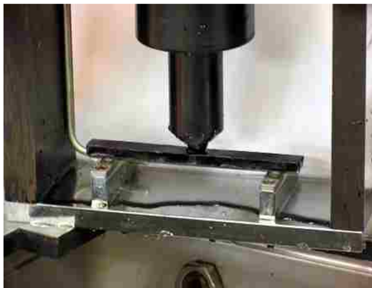
Figure 8: BBR beam on its supports [26]
