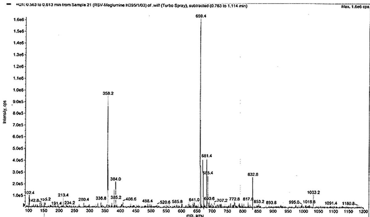
Fig. 10. ESI (+ve) mass spectrum for adduct impurity.
