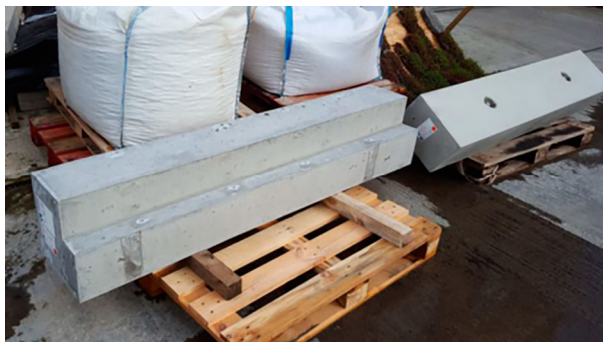
Figure 6. Precast concrete beam cast for upscaled testing.
