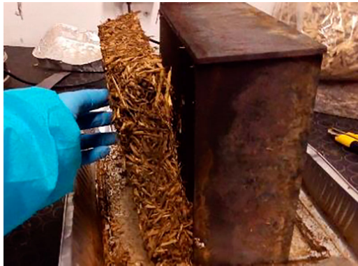
Figure 5. Insulation panel made from wood fibres.
