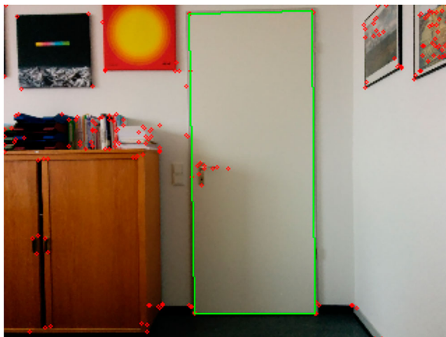
Figure 8. Example of the detected door. The red dots are corner points and the green rectangle is the correctly detected door.
