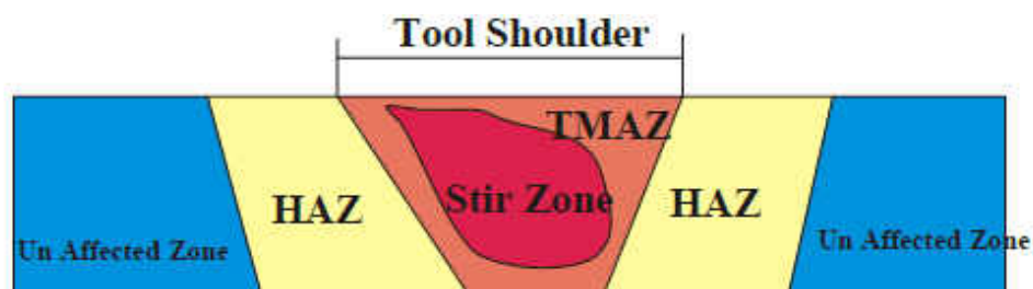
Figure 2-27: Various zones generated in the FSW process [85]
