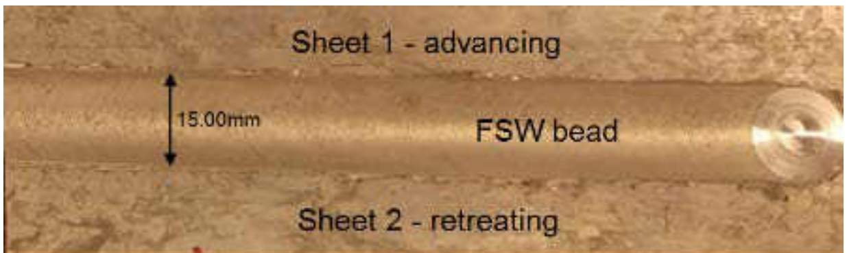
Figure 3-2: An example of a successful FSW joint produced in this study (1200 RPM, and 420 mm/min).
