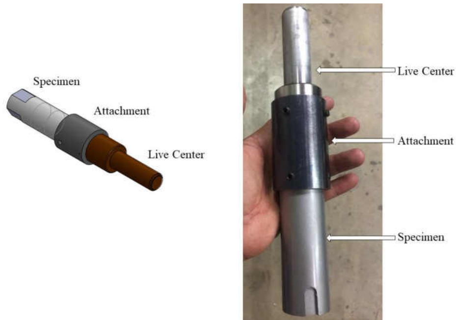
Figure 4.30 Assembly of Live Center, Attachment and Specimen. (Left) 3D Cad Model (Right) Manufactured attachment in assembly.
