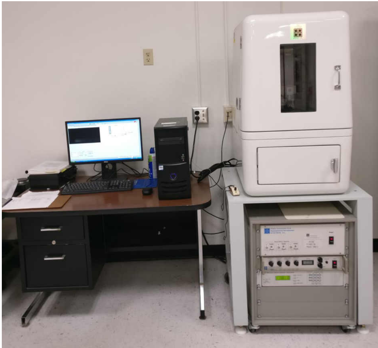
Fig. 3.3: Hysitron Ubi-1 Nanoindenter used in this project.
