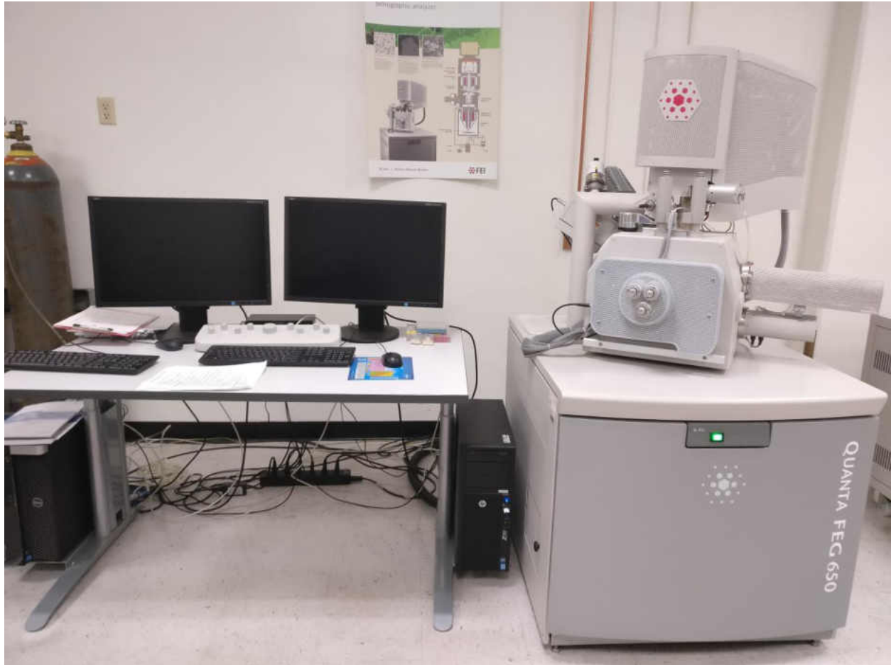
Fig. 3.7: QUANTA FEG 650 Scanning Electron Microscope used in this thesis.
