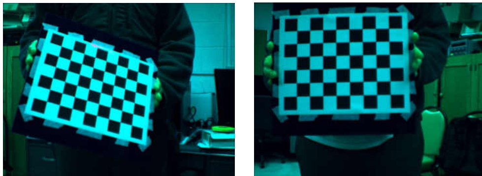
Figure 34. Calibration images used for the Tetracam ADC lite camera calibration
