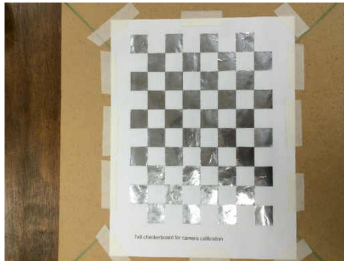
Figure 37. Calibration Checkerboard pattern made with aluminum foil sheet and paper
