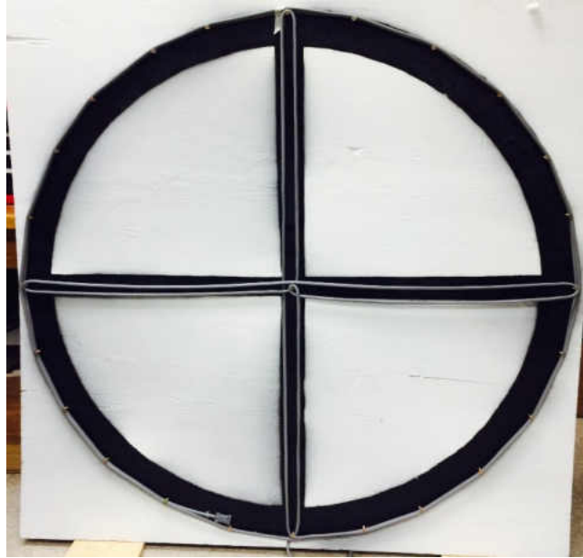
Figure 24. Target board for tuning the camera alignment. Black markings are the enamel paint and the gray heating wire is wrapped around the path of the painted enamel.
