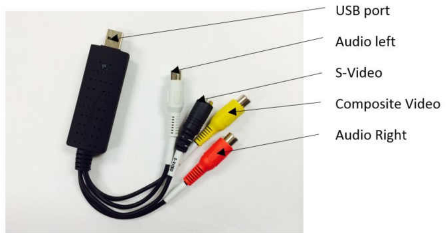
Figure 10. Sabrent USB-AVCPT 2.0 Video/Audio Capture & Converter
