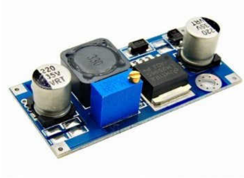
Figure 12. DC-DC step-down voltage regulator [39]
