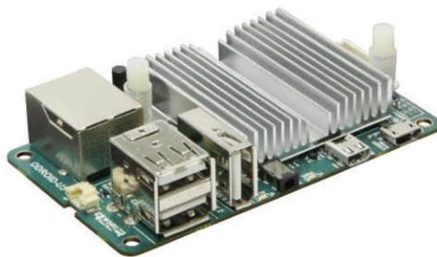
Figure 9. Odroid U3 single board computer [37]
