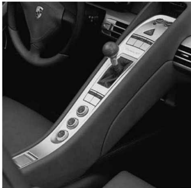
Figure 2-25. Highlights one successful application of magnesium in producing center console cover in Porsche Carrera GT [16].
