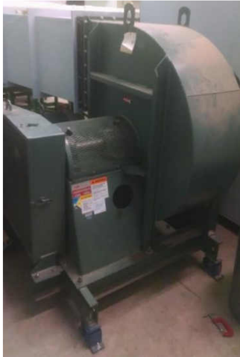
Figure 2. New York Blower used for Wind Tunnel
