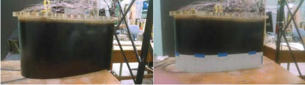
Figure 18. Painted heat transfer vane (left) painted vane with dot location grid (right)
