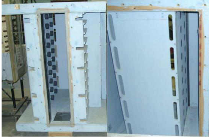
Figure 10. Exit of mock aero combustor (left) and inlet of mock aero combustor (right) [42]
