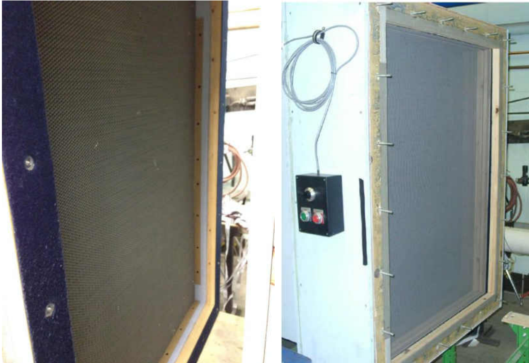
Figure 5. Flow straightener (left) and screenboxes (right).
