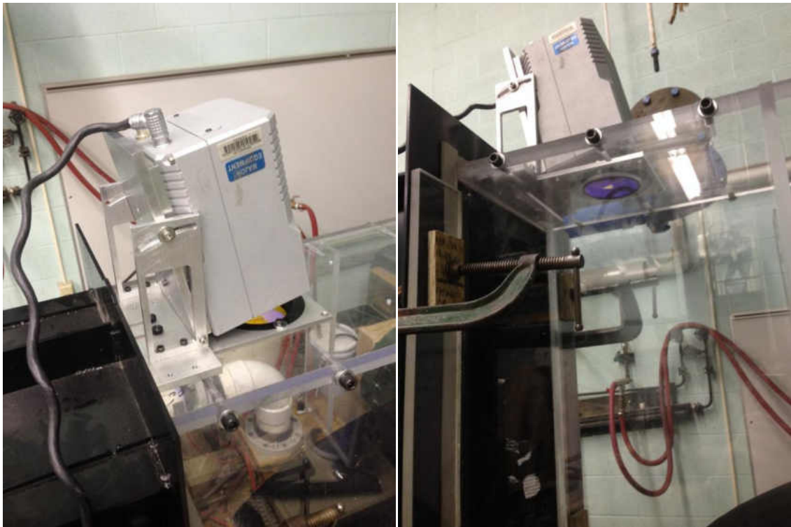
Figure 20. Mounted IR camera and zinc selenide window.
