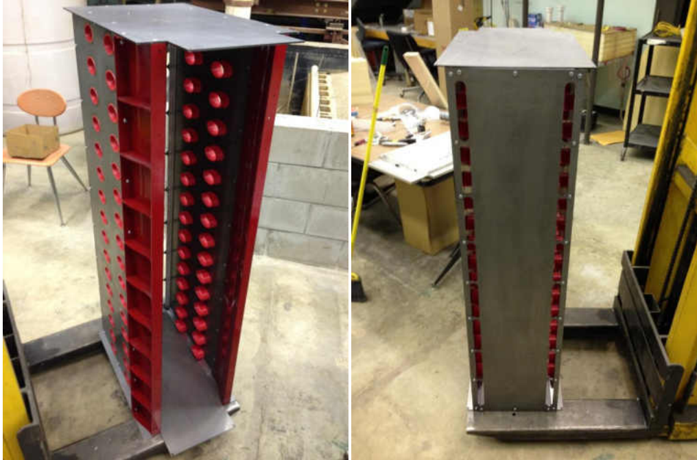
Figure 31. Photos of completed turbulence generator mock liner.
