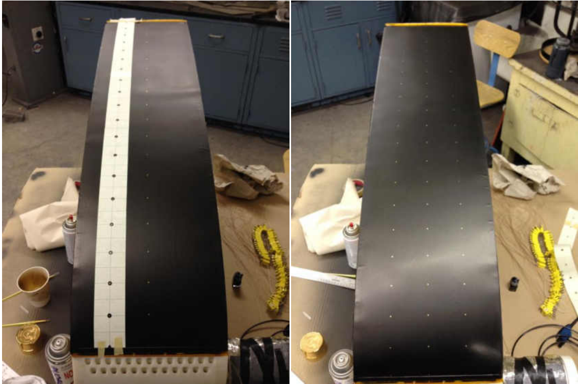
Figure 21. Painted test surface with gold dot jig (left) and completed surface (right).
