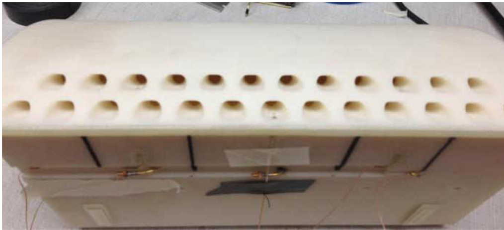
Figure 15. Instrumentation in shaped holes insert.
