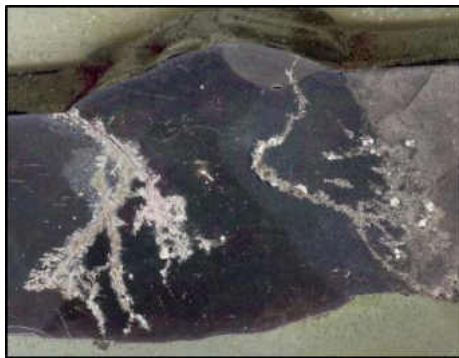
Figure 1.7: Liquid metal embrittlement failure on brazed aluminium heat exchanger [52].
