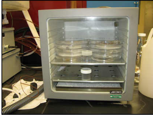
Figure 2.5: EERC Desiccator used to keep filter samples.
