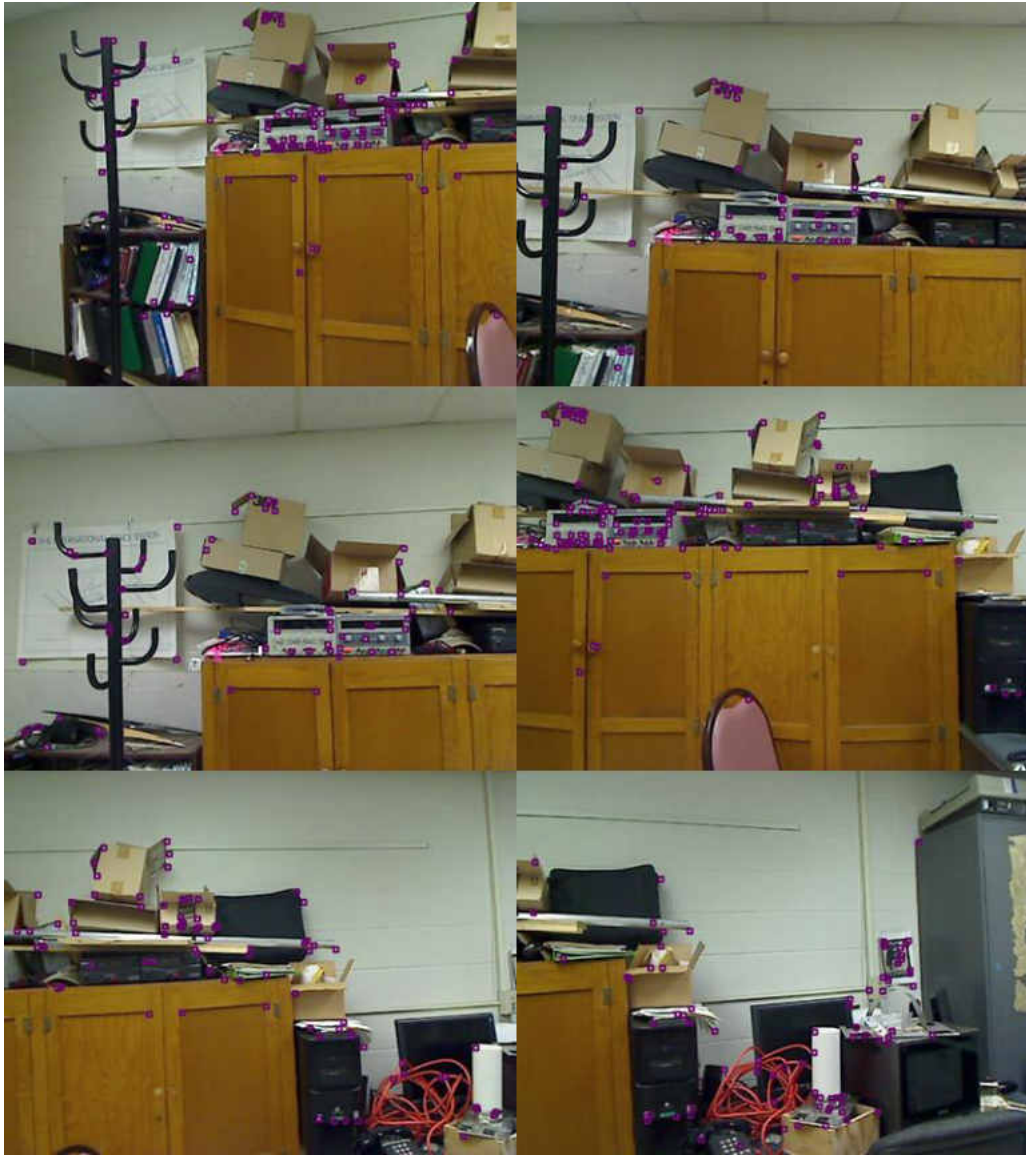
Figure 16: Few snap shots of the environment where the SLAM algorithm was run. The pink dots represent the map points that are successfully tracked for camera pose estimation.
