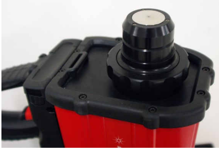
Figure 9: Attenuated total reflectance (ATR) attachment for Agilent 4100 ExoScan
