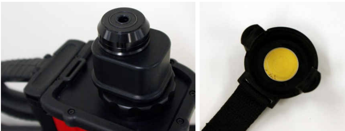
Figure 14: (Left) Diffuse reflectance attachment (Right) reference sample cap for Agilent 4100 ExoScan
