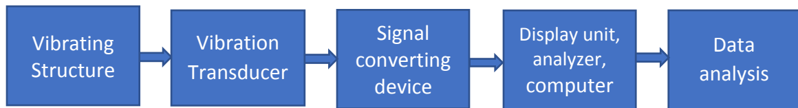
Figure 1.1: Basic vibration measurement scheme
