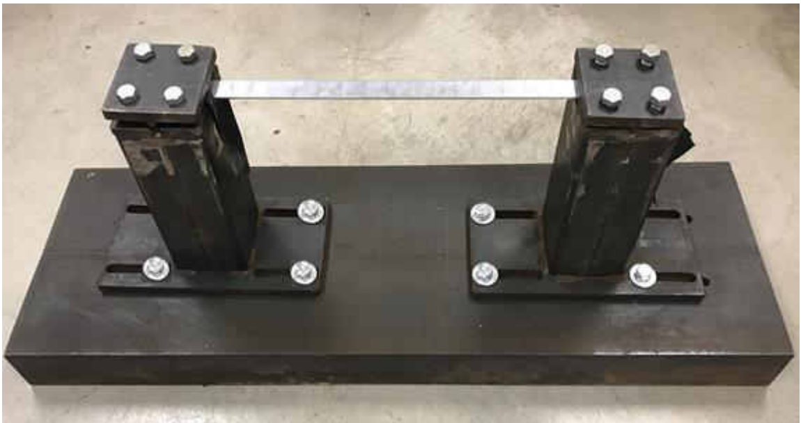
Figure 4.2: Setup for Simply Supported boundary condition of the beam.
