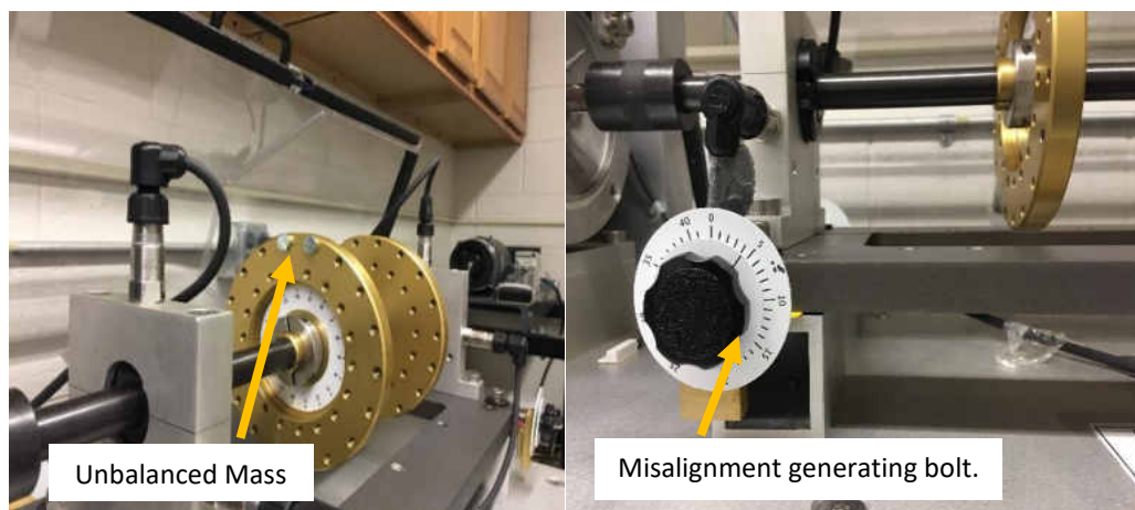
Figure 2. 4 Unbalanced and misaligned condition simulation.
