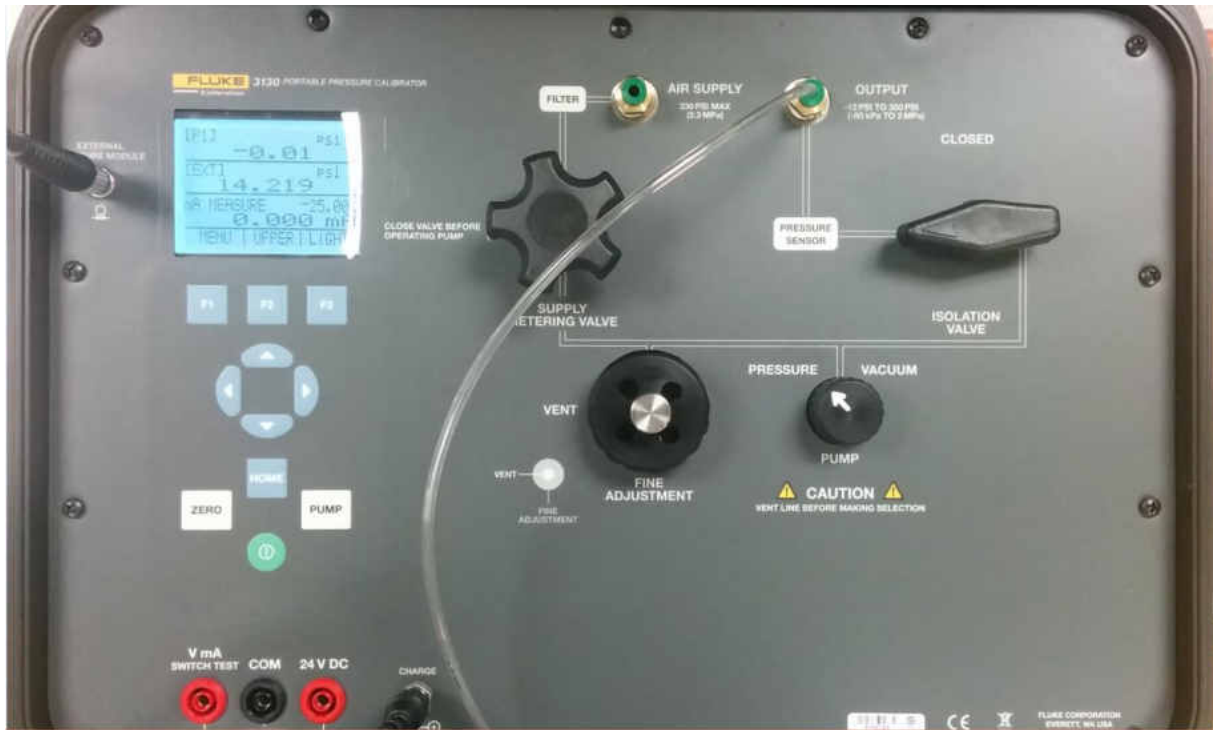
Figure 44: Fluke pressure calibrator used to calibrate the Honeywell PX2 pressure transducers.
