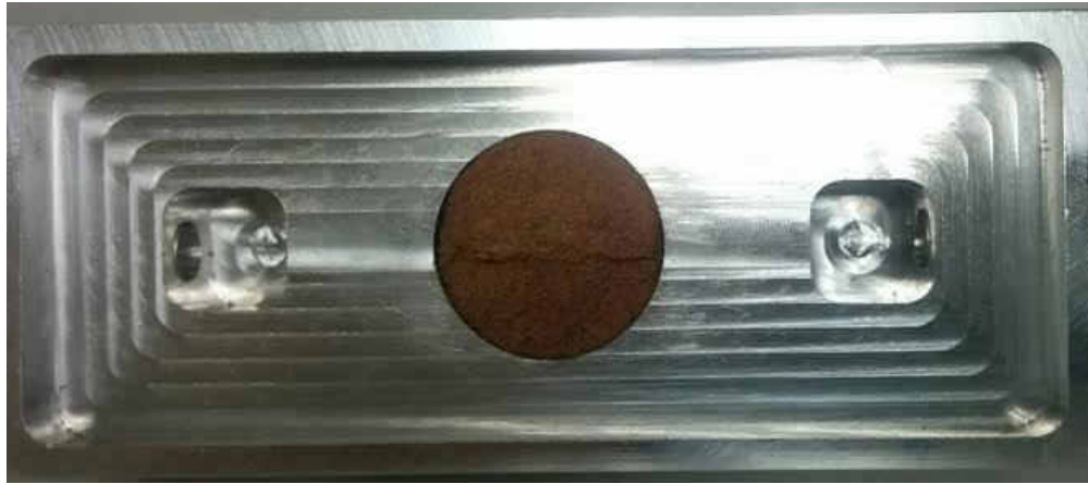
Figure 36: Base section with porous media inserted into testing slot
