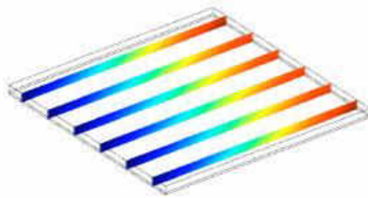
Figure 24: Temperature distribution of porous media microchannel (Lim et al., 2010).
