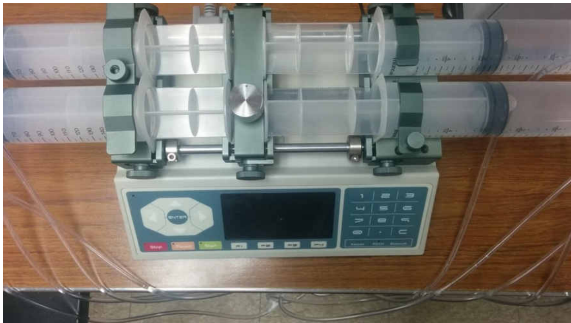
Figure 31: Nexus 3000 syringe pump with optional continuous flow rack and four 140 mL Monojet syringes installed
