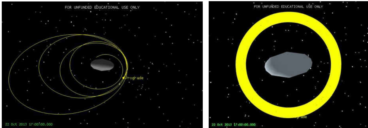
Figure 40. Example of an unstable prograde orbit and a stable retrograde orbit. Both orbits shown have the same initial conditions, but are separated by 180^\circ of inclination.
