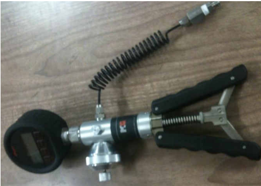
Figure 31. Ametek hand pump for calibration of the pressure transducers.
