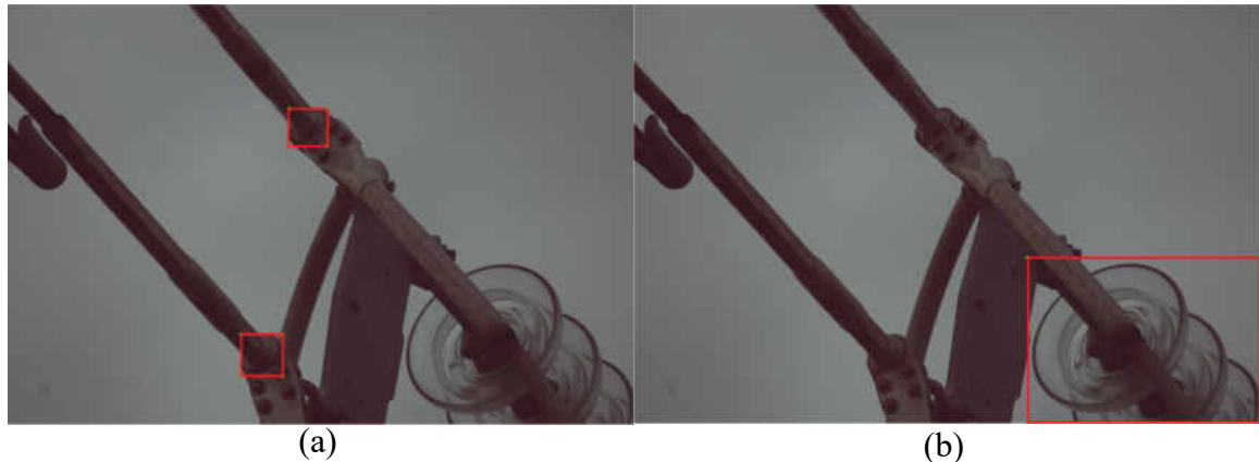
Figure 16: Example images of bounding box annotations for one image (a) DEBC welds (b) insulator
