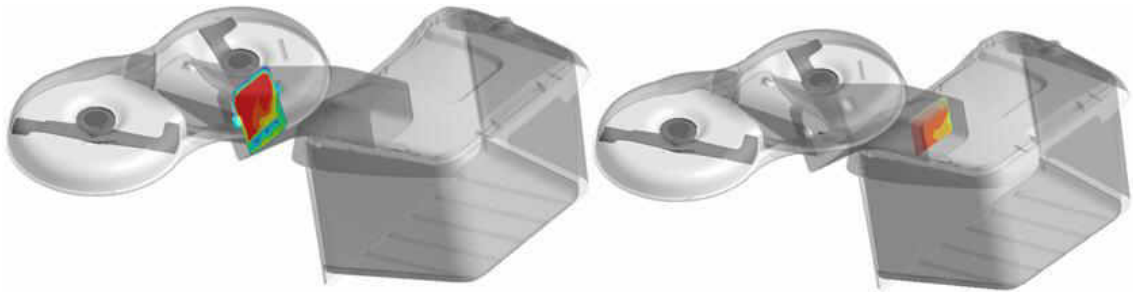
Figure 22. CFD flow field locations within the MCS chute. The one on the left being the deck chute nozzle exit and the one on the right being near the exit of the MCS chute.
