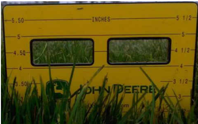
Figure 30. Grass height gage showing uncut grass to be about an average of 3.25 inches.
