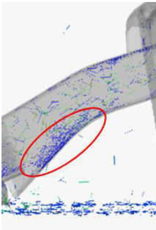
Figure 34. Beginning stages of material buildup in the B1 model discharge chute.
