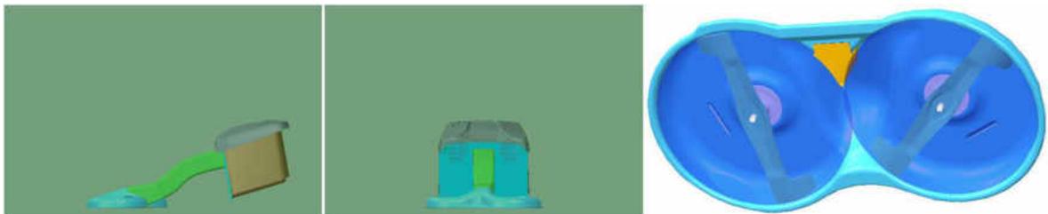
Figure 50. CFD bounding box and mower blade control volumes.
