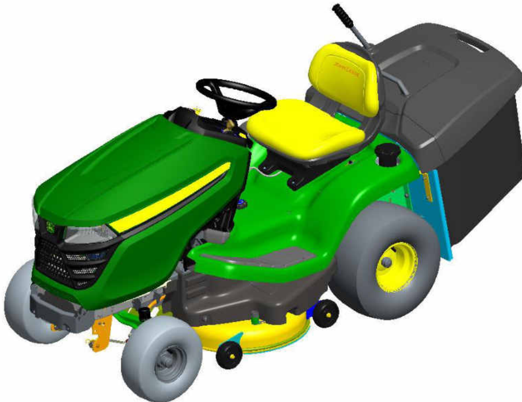
Figure 1. CAD model of the John Deere Select Series X350R Model Year 16 Tractor. This is a typical looking dedicated RDRC unit.
