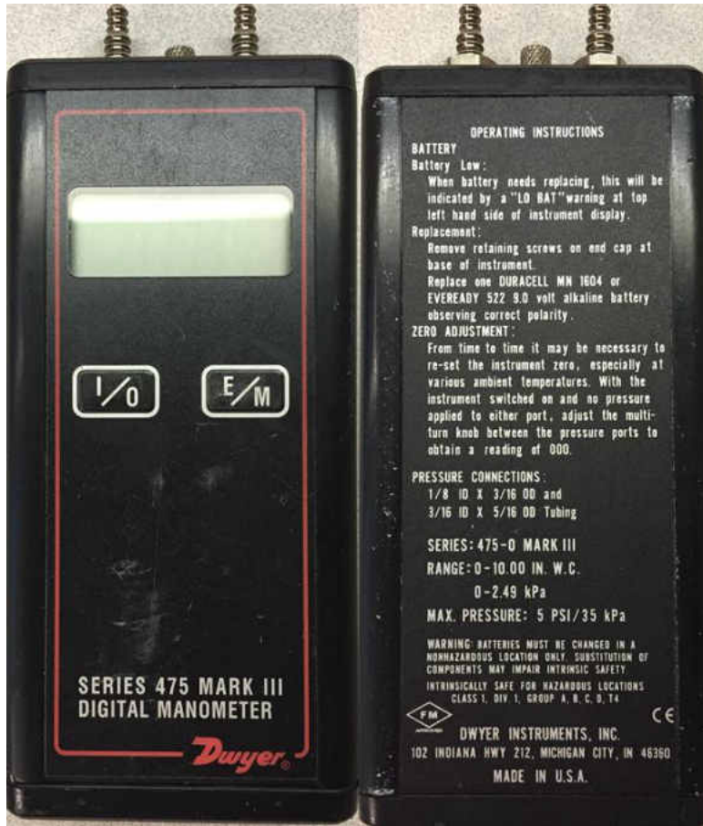
Figure 19. Dwyer Instruments, Series 475 Mark 3 Digital Manometer. This manometer has a range of 0 – 10.00 Inches of W.C. (water column) or 0 – 2.49 kPa.
