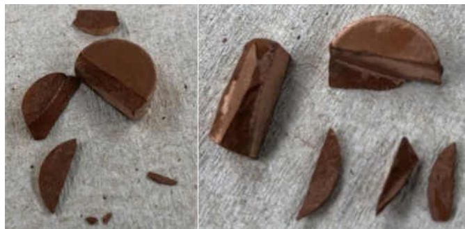
Figure 2.2: Fractured copper samples fabricated at 300 °C.
