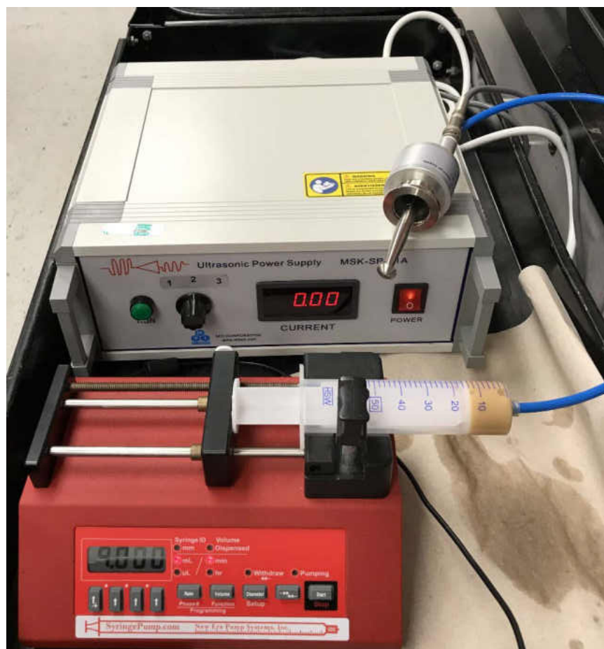
Figure 5.1: Atomizer nozzle attached to an ultrasonic power supply and syringe with a syringe pump.
