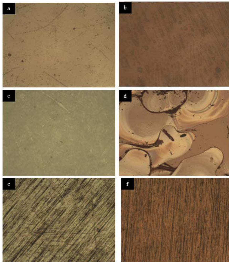
Figure 4.2: Optical microscopy at 10X magnification of (a) as-received mica, and (b) lignin-acetone coated mica (c) as-received Corning glass, (d) lignin-acetone coated Corning glass, (e) as received stainless-steel, and (f) lignin-acetone coated stainless-steel.
