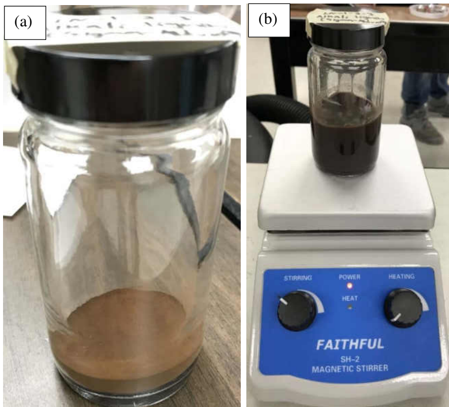
Figure 2.1: (a) 5 g of lignin in a glass container, and (b) lignin particles in acetone (before stirring).
