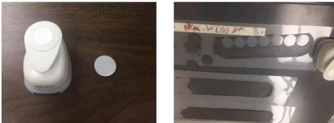
Figure 2.4: (a) Punch die used for fabricating 1" samples, and (b) examples of laminates after
