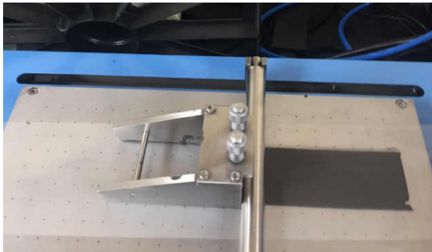
Figure 2.2c: Tape casting set up for casting individual layers
