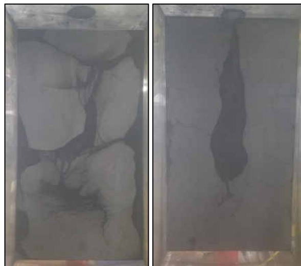
Figure 33: Poor Fluidization Regime (left) vs Optimal Fluidization Regime (Right) – 94 micron OC
