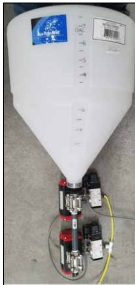
Figure 27: Double Dump Valve system set up
