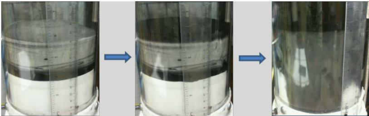
Figure 11: Traditional fluidization regime control test showing carbon mixing behavior (left to right)
