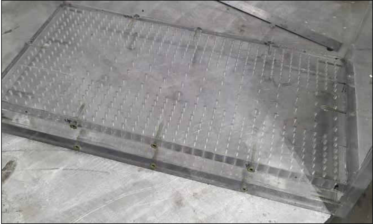
Figure 21: Distributor Plate for Large Char Separator
