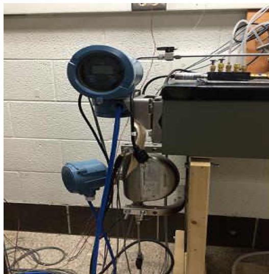
Figure 3.4 Micro Motion mass flow sensor connected to a 1700R model transmitter.
