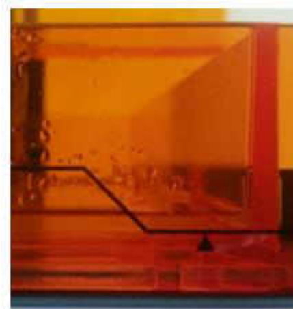
Figure 1.8: An indicator mark showing minimum threshold level in a 3D printer
