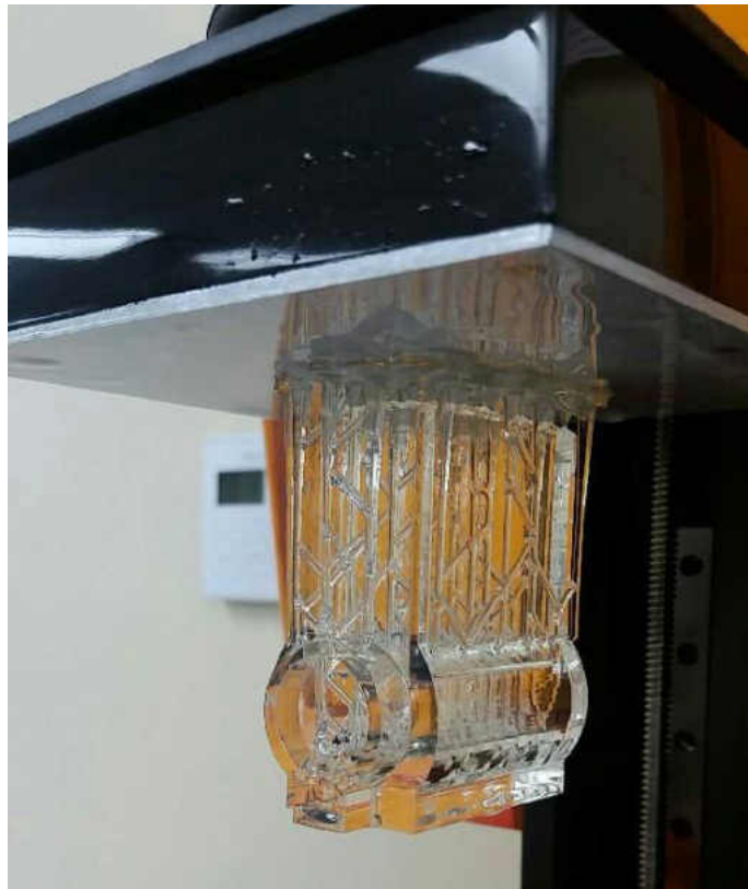
Figure 1.11: A picture of the hopper 3D printed by Form 1 lab
