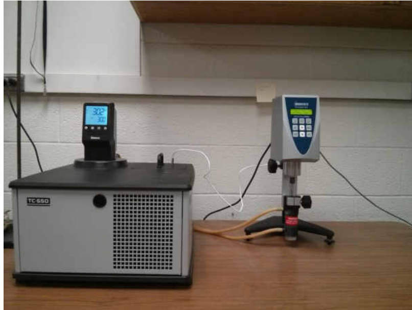
Figure 3.3: DV II+Pro Extra Brookfield viscometer connected to the TC-550MX temperature bath
