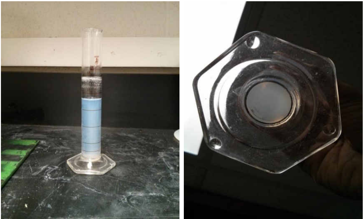
Figure 3.1: Sample of prepared 20% by mass silica nanoparticle suspension after 30 days of preparation
