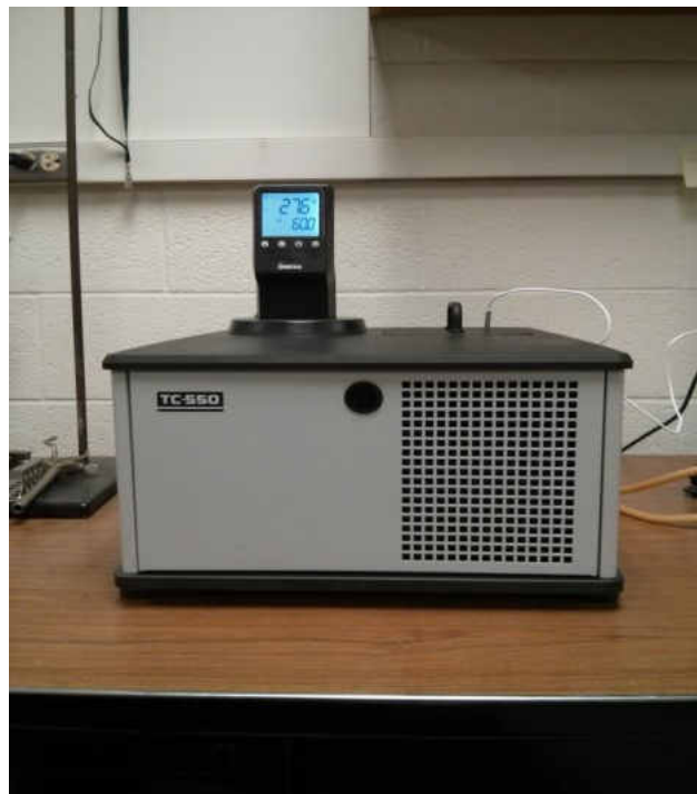
Figure 3.2: TC 550MX constant temperature bath
