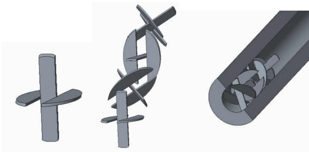
Figure 34 Triple Plate (a) single element (b) element chain (c) static mixer
