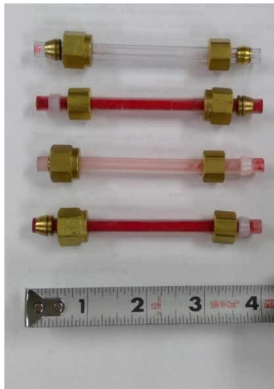
Figure 71 Static mixer test section tint after experimental tests arranged from top to bottom: empty pipe, helical, double plate, triple plate
