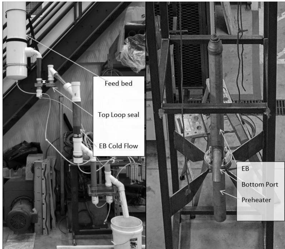
Figure 13. Cold flow EB unit (left) and hot flow EB unit with air preheater (right)
